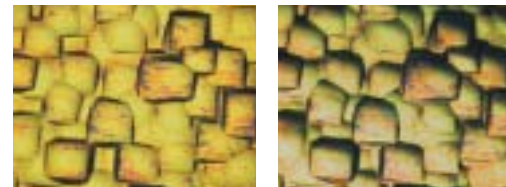
Surface of metal chips at 1700x magnification.
