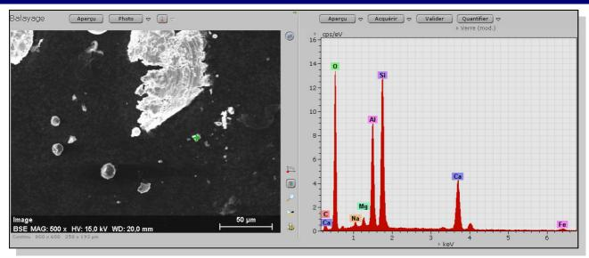
Esprit Software (EDS Bruker XFlash): selective analysis on micrometric particles.
