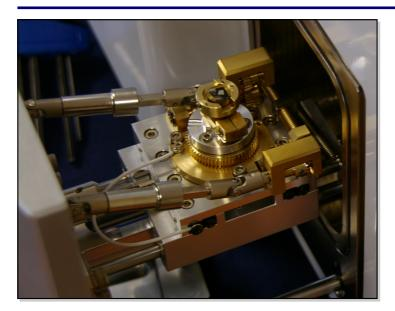
3 axis table: X, Y, R and movement 20 \* 20 mm /  $360^{\circ}$
